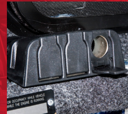
THREE-OUTLET 12- VOLT POWER BLOCK
