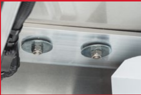
Bolt Plate Reinforcement for Aftermarket Rack System (Optional; Required with all Commercial Rack Options)
